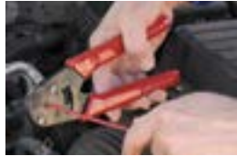
Crimps Closed Barrel Deutsch Terminals
