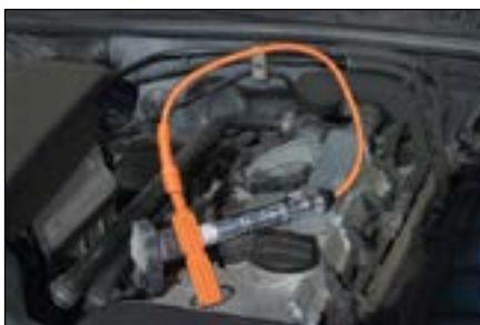
Test vehicles with recessed spark plugs
