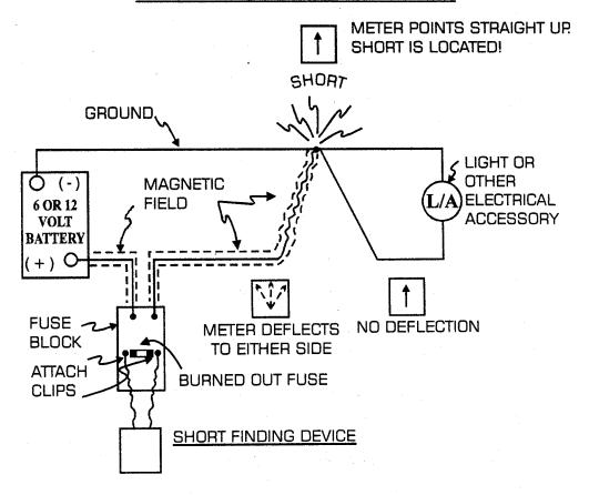
NOTE: BEFORE USING THIS DEVICE, CONSULT THE VEHICLE SERVICE MANUAL FOR SPECIFIC CIRCUIT DIAGRAMS IN EACH FUSED CIRCUIT AND ANY PARTICULAR TEST OR REPAIR PROCEDURES. NOT RECOMMENDED FOR TESTING ELECTRONIC ENGINE OR BODY CIRCUITS INCLUDING: COMPUTERS, SENSORS, FUEL INJECTORS AND AIR BAGS.
