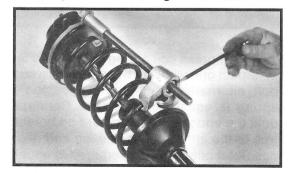
**4.** Be sure that movable hex nuts are threaded onto bolt and seated in hex holes of double hook as shown. Hand tighten bolt.
