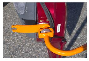
Open vehicle door. Slide Insert Pin into the open door latch until it completely locks.
