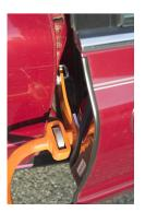
Rotate Knurled Drive Nut clockwise until the Heel is flush with the door. Do not over tighten.
