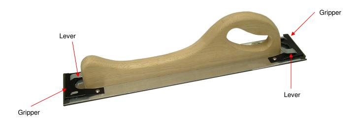
Have a  $2\frac{3}{4}$ " x  $17\frac{1}{2}$ " standard cut abrasive sheet. Raise one lever so it is at a right angle to the base. Insert the sheet of sandpaper under the gripper. Return the lever to the original position. Raise the second lever so it is at a right angle to the base. Wrap the sandpaper around the bottom of the base under the second gripper. Return the second lever to the original position.
